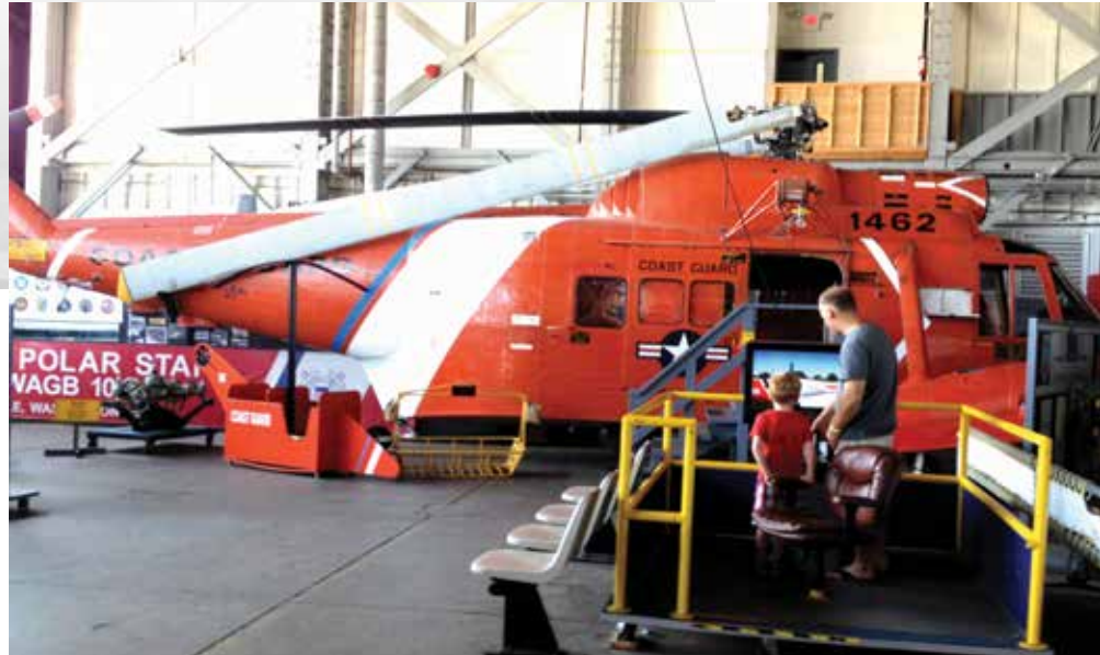
The Sikorsky HH-52 Seaguard was a single turbine engine, three-blade rotor amphibious helicopter was used by the United States Coast Guard primarily for air-sea rescue.
